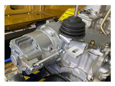
The GT-LT95 overdrive gearbox takes advantage of Global Roamer's legendary epicyclic gear train technology which is used in their ROAMERDRIVE overdrive gearboxes. Also known as *planetary gear sets*, they are well known for their strength and durability. Global Roamer Corporation has a world-wide population of many thousands of overdrives using this very same *bullet-proof* technology.
