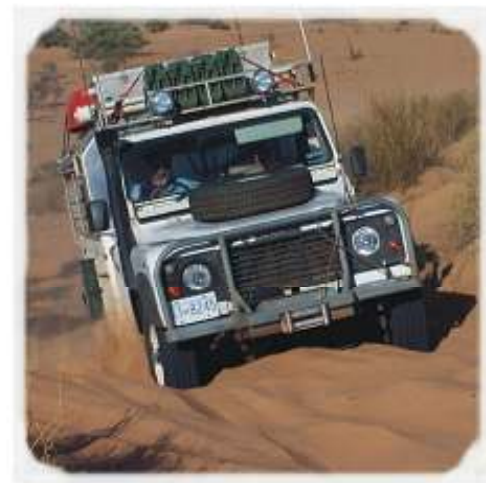
The pictures show the same Defender 110 in high range overdrive on the Gunbarrel highway (left) and in low range climbing 'Big Red' a major dune in the Simpson Desert. (above) Momentum accrued between dunes allows the Land Rover to gain ground up the dune face where it might otherwise bog down in sand. Pictures are from a test expedition in Australia.
