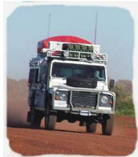
The pictures show the same Defender 110 in high range overdrive on the Gunbarrel highway (left) and in low range climbing 'Big Red' a major dune in the Simpson Desert. (above) Momentum accrued between dunes allows the Land Rover to gain ground up the dune face where it might otherwise bog down in sand. Pictures are from a test expedition in Australia.
