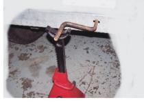
To do this engage first gear, insert the hand crank into the engine, and block it to stop rotation. The nut can now be tightened to a torque of 110 lb/ft (135N/m).
