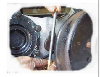
Attach the dip stick tube to the elbow and tighten firmly. Note that the tube passes over the nut securing the end of the lay shaft. The speedometer cable passes between the dip stick tube and the aft side of the transfer case.
