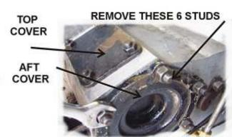
Remove the six nuts holding the round PTO cover and the four nuts holding down the transfer case top cover. Both covers can be stored as they are no longer required. The four nuts and washers for the top cover will be re-used and the four studs are left in place. The six studs that held the aft cover must be removed. A vise-grip can be used for this purpose or two nuts locked together.
