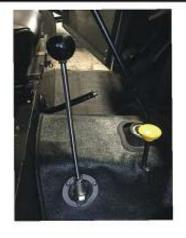
Before using the overdrive make sure that no part of the lever, 'L' bracket or tie rod contacts any part of the Land Rover bodywork, panels, screws etc. Such contact will cause noise and vibration in the cab. The upper RH screw that holds the tunnel cover may need to be shortened. In some installations you may have to bend or twist the 'L' bracket to get comfortable bodywork clearance.
