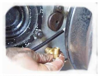
Start by installing the dipstick bushing and elbow. Separate the dipstick tube from the brass elbow and screw the elbow into the filler plug orifice using a sealer such as 'Permatex'. Stop when the elbow is tight and pointing up towards the lay shaft immediately above it.
