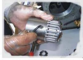
screws on the periphery of the coupling are sitting flush with the outer surface. Remove the hexagon nut from within the cupling.
