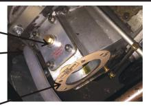
Using the rectangular gasket provided, secure the new aluminum top cover in position using a gasket sealant. Fit the new hexagon socket filler plug.
