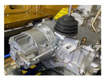
The GT-LT95 overdrive gearbox takes advantage of Global Roamer's legendary epicyclic gear train technology which is used in their ROAMERDRIVE overdrive gearboxes. Also known as *planetary gear sets*, they are well known for their strength and durability. Global Roamer Corporation has a world-wide population of many thousands of overdrives using this very same *bullet-proof* technology.
